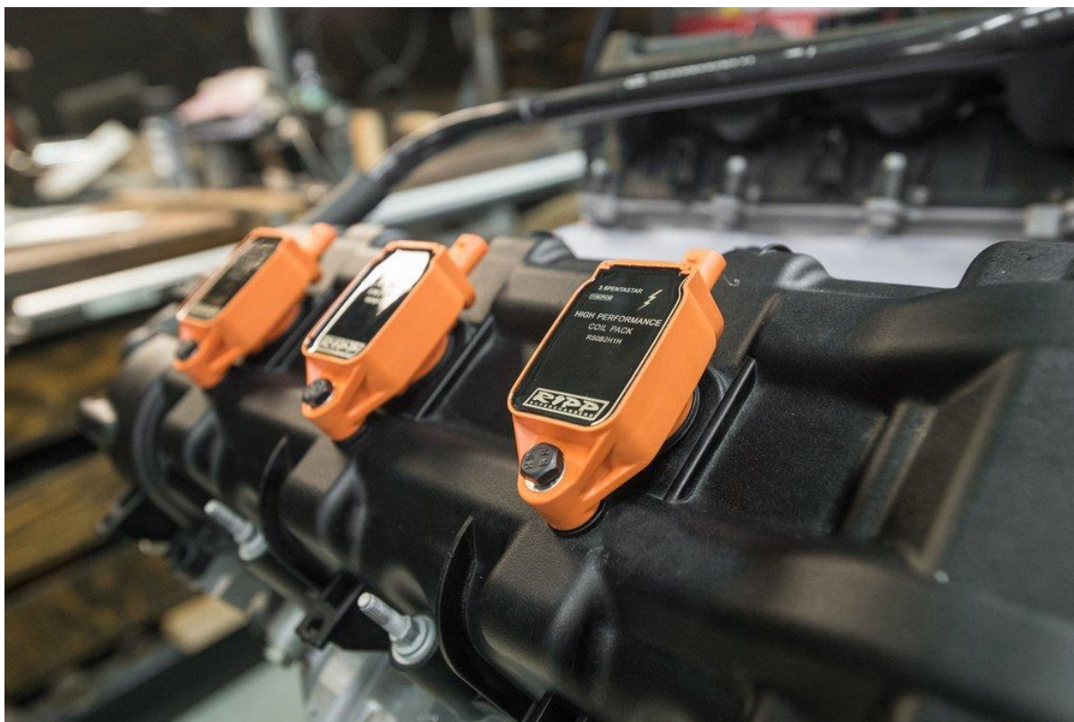
ECU-electronically controlled coil packs. (Photo: Rippmods.com)
