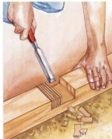
Start the notches with a series of saw cuts, then remove the material with a sharp wood chisel.
