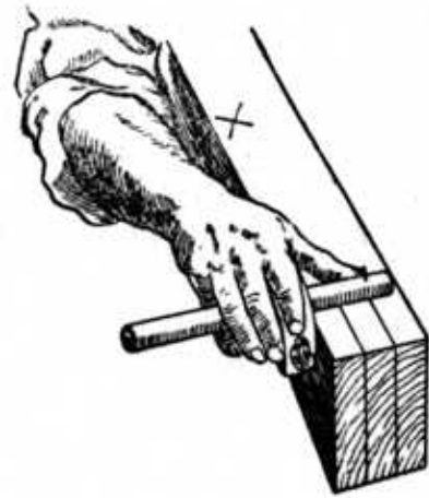
Fig. 82.—Gauging the Timber.
