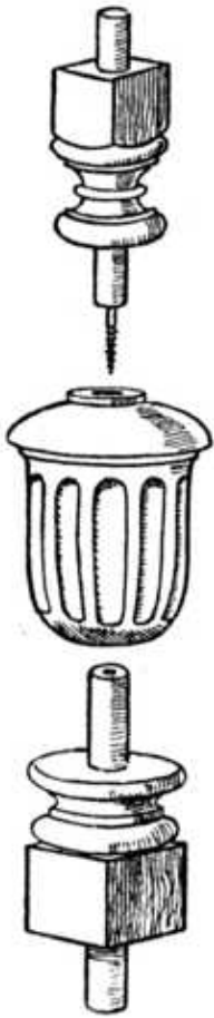
Fig. 349.—Method of Building up Turnings.
