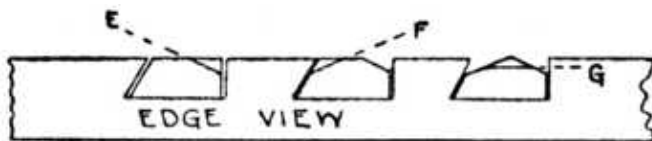
Fig. 319.—Showing Method of Paring.
