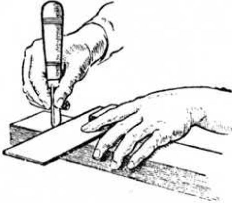
Fig. 64.—Marking the Joint with Try Square.
