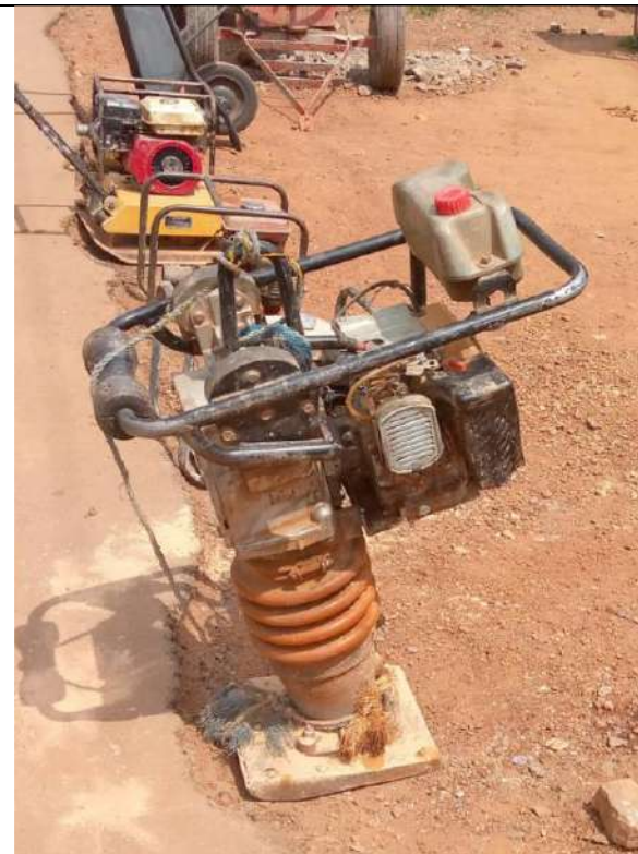
JUMPER COMPACTOR CONCRETE MIXER
