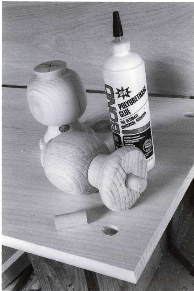
Use 3/4" dowel and one of the new polyurethane glues to fasten the feet to the kicker.
