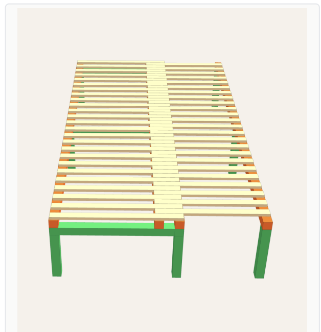
Comb open — the mobile part (battens 2/4 + every other slat) slides out to double the bed's width.
