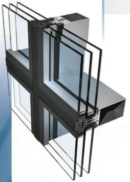
Non-frame curtain wall with the structural glazing assigned for the realization of lightweight facades and other spacial constructions. The post-transom construction of PF 152 system is used as a load bearing element. The external side of PF 152ESG is uniform, smooth glass wall divided with vertical and horizontal lines at width of 22 mm using weather silicon or at width of 28 mm using the closing gasket. There is a possibility of assembling double and triple glazed units.
