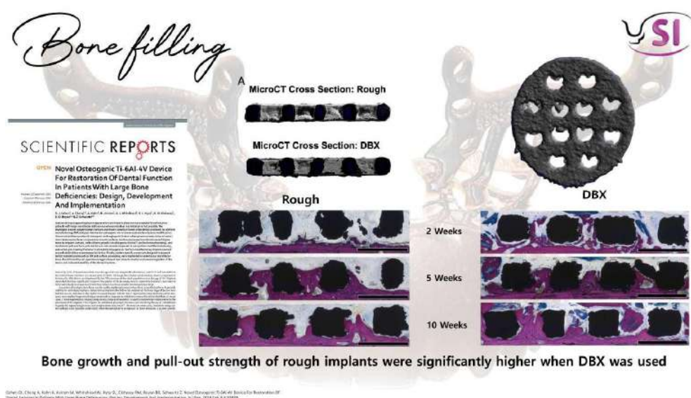
Figure 9.3 — Bone ingrowth and pull-out strength significantly higher with DBX coverage. Rough + DBX group shows markedly superior bone volume (BV/TV%) at 5 and 10 weeks, and highest pull-out force at week 10. The biomaterial acts as both biological stimulant and spatial maintainer. Adapted from Cohen and al. 2016.
