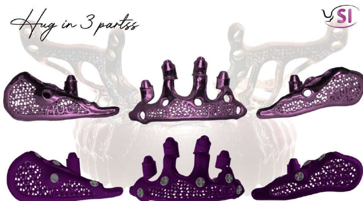
Figure 15.45 — Three-part HUG® implant design (bottom row) and the resulting titanium SLS-printed components (top row).
