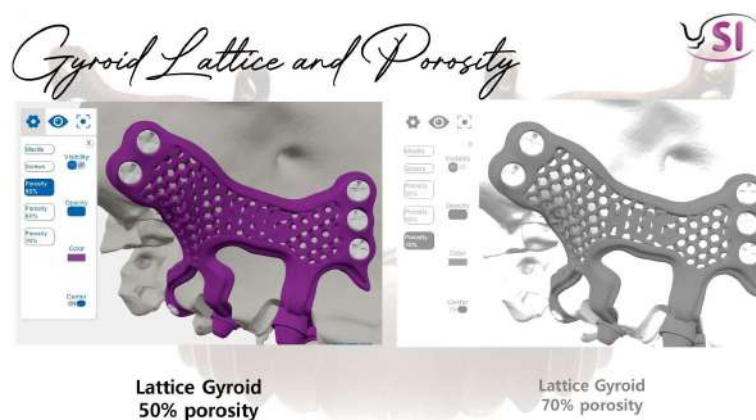
Figure 4.4 — Comparison of Gyroid Lattice designs at 50% and 70% porosity on a maxillary HUG® implant. The 50% version delivers the optimal balance between biological performance and mechanical strength; the 70% version was rejected following biomechanical validation.
